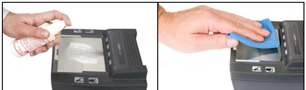
Figure 4.1 Cleaning with glass cleaner
