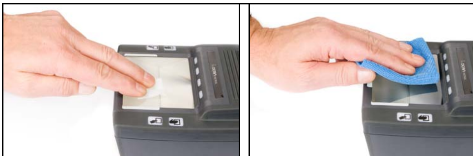
Figure 4.2 Cleaning with Alcohol Prep Pad
